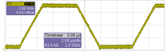
Fig. 9. The VCO tuning voltage transient when f_{ref} switched from 5900 MHz to 6900 MHz.
